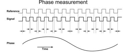
**Fig. 1.** Phase is measured by periodically timing the difference between a reference and the signal and plotting this difference over time.
